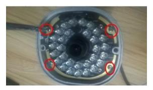
**Step3**: Carefully take out the whole lens board, please find the SD card slot on the inside PCB;
