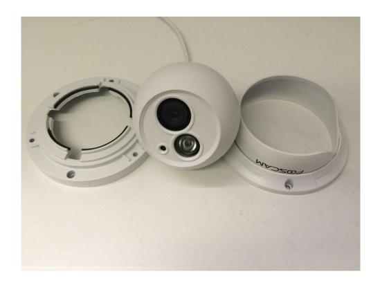
Unscrew the top and bottom of the dome to open the camera and access the Micro SD Card slot.
