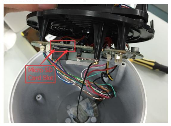
**Note**: Please make sure to screw up the camera in case of the Lens will scratch the dome when pan/tilt and the water entering when you place it outside.
