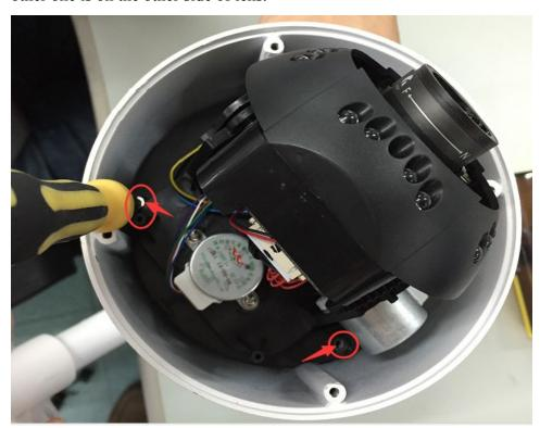
**Step3**: After taking off the three screws, please take the Lens part away slowly in case the cable inside the camera is broken.
